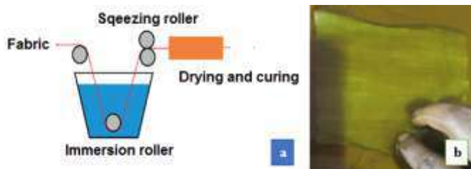
Figure 2: a. Pad-dry-cure method and b. Coated sample
