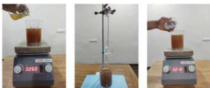
Figure 1: Microcapsule preparation a. Extract of TP, b. adding Sodium alginate, c. adding nontoxic binder
