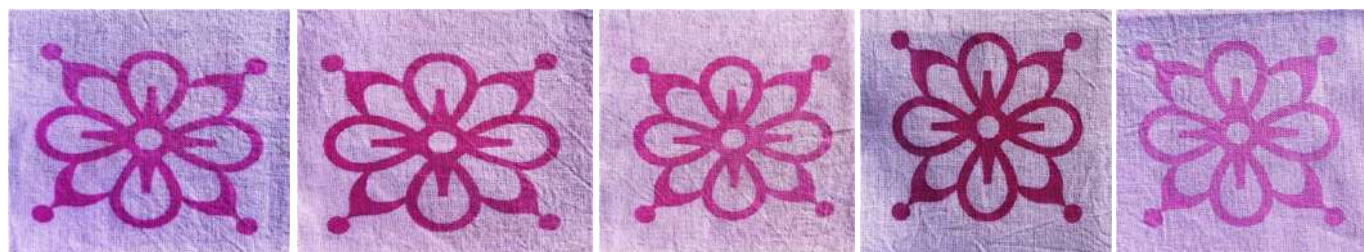
Sodium alginate Thickener Unmodified flaxseed thickener Modified with ZnO Modified with acrylation Modified with TiO2
