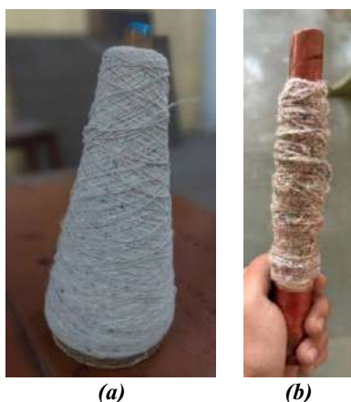
Figure 1 - Prepared Yarn Samples a) Rotot-Spun Yarn b) Ring-Spun Yarn
