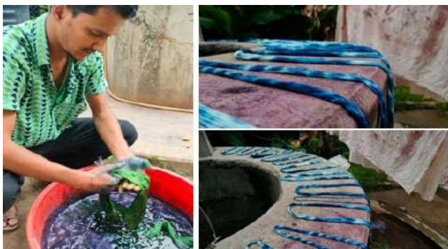
Figure 3: Dyeing of weft yarn using natural Indigo
