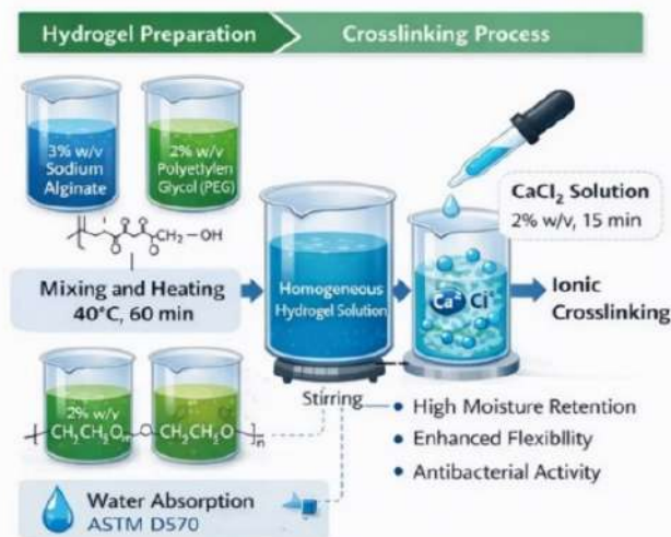
Figure 1: Hydrogel synthesis and crosslinking process schematic
