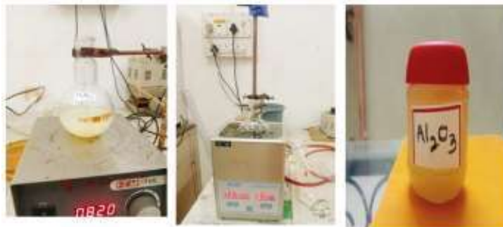
Figure 2: Synthesis process of Al_2O_3 nanofluid using coconut oil and Oleic Acid
